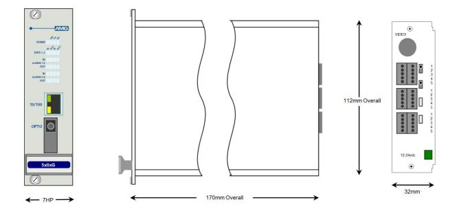
The **AMG5902HPG** is a rackmount Ethernet Media Converter receive unit designed to provide 100BASE-TX full duplex Ethernet connectivity over one singlemode fibre. The HP suffix in the partno. indicates High Power optical transceivers.
